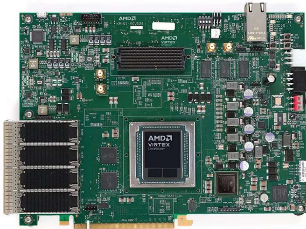
AMD Virtex™ UltraScale+™ HBM VCU128 FPGA Evaluation Kit
