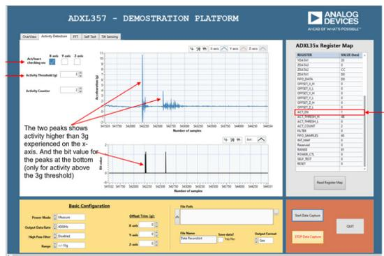
Figure 17. Activity Detection for X-Axis
