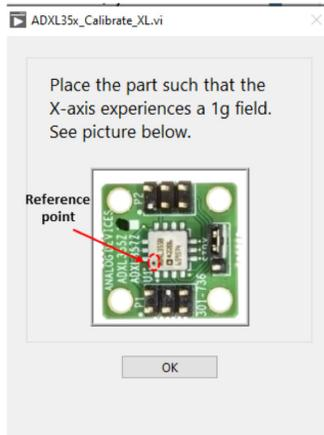
Figure 22. +1 g Calibration (Orientation for X-Axis)
