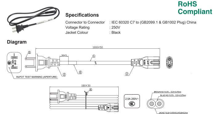
INDENT MARKING : (C A003145 60227 IEC 52(RVV) 300/300V 2X0.75mm 2
