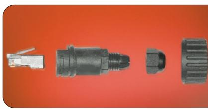
between each connection point. The RJ-Lnxx\* field attachable connector enables bulk cable to be pulled to the exact required length, and then terminated to the RJ-45 plug using readily available crimp tools. The completed assembly provides the same sealed, robust connector as the RJ-Lnxx overmolded cordset.
