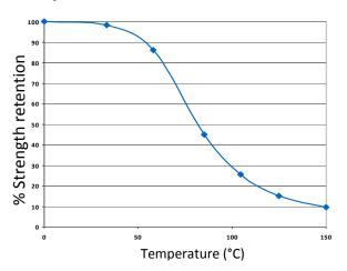
ET500 can withstand higher temperatures for brief periods (such as for paint baking and wave soldering processes) providing the joint is not unduly stressed. The minimum temperature the cured adhesive can be exposed to is -40°C (-40°F) depending on the materials being bonded.
