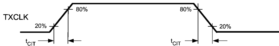
FIGURE 2. Transmit Clock Transition Times
