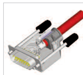
Mount connector and cable into the backshell
