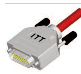
Assemble the other half (screwing force: 100-120 Ncm)
