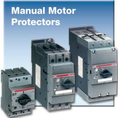
A broad range of units available to protect 3-phase motors up to 100 A/75 HP. UL listed and CSA certified for group motor installations and self-protected combination motor controllers. Short-circuit protection, adjustable overload protection, and manual disconnect capability. Common bus bars, auxiliary contacts, and many other standard accessories available.
