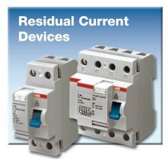
Residual current devices provide equipment protection from fires and electrocutions caused by ground faults. These compact units feature DIN rail mounting and are available in a wide array of thresholds: 10, 30, 100, 300, and 500 mA. UL, CSA, IEC, CE, and many other agency approvals.
