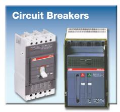
Ideal for all electrical power generation and distribution applications. Isomax molded case circuit breakers, UL/CSA rated 600 VAC, feature continuous currents from 15 A to 2500 A. Emax power circuit breakers, UL rated 600 VAC, operate with continuous currents to 5000 A. Extended working life of all internal parts ensures high reliability and continuous operation.
