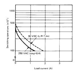
Note: The service life graphs apply to all relay output models. They do not apply to solid-state output models H5CN-XZNS or H5CN-XANS.
