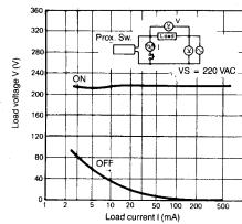
Note: When the current rating of the load is less than 10 mA, false operation may occur. This is normal, and the problem can be solved by installing a bleeder resistor in parallel with the load. Use the formulas given here to calculate the power rating and value of the resistor.
