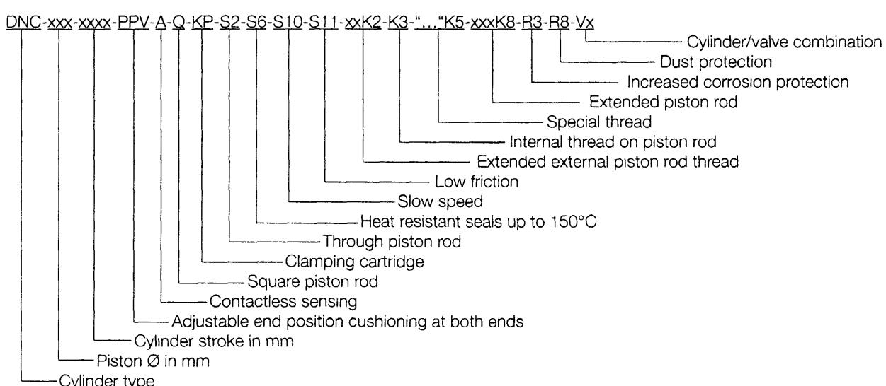
**How to order:** Type + piston Ø + stroke + adjustable end position cushioning + sensing + square piston rod + through piston rod + extended piston rod + heat resistant seals
