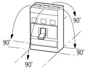
With residual–current release NZM1, N(S)1: Vertical and 90  $^\circ$  in all directions
