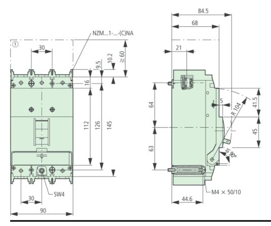
Clearance from conductive parts 60 mm
