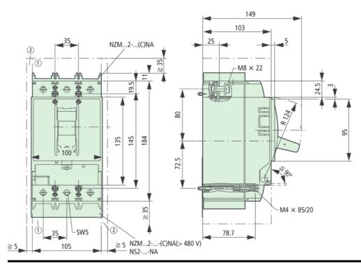
Clearance from conductive parts 35 mm, laterally 5 mm
