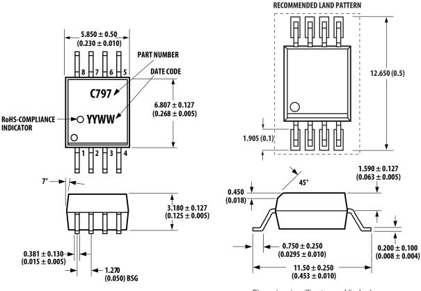
Dimensions in millimeters and (inches). Lead coplanarity = 0.1 mm (0.004 inches).
