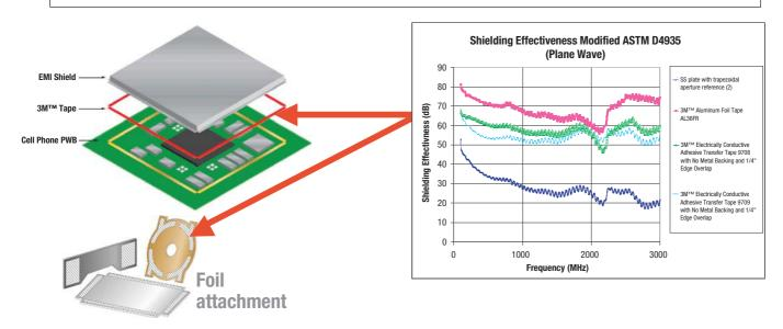
3M<sup>™</sup> Electrically Conductive Adhesive Transfer Tapes 9703, 9705, 9706, 9708, 9709, 9709S, 9709SL, 9712, 9713, 9714, 7805 and 7810 can provide FPC grounding and tapes 9708, 9709, 9709S, 9709SL, 7805 and 7810 can increase the effective EMI Shielding through the bond line thickness leading to improved product EMI Shielding performance of the FPC.
