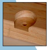
Uniquely the MAD-bit can form a "flat bottom" hole which, in one single action, facilitates the fitting of 1" (25mm) recessed hinges as installed in kitchen cupboard doors and many RV and caravan furniture fixtures. (This task previously required the use of a specialised recess tool). All other conventional drill bits form a pointed hole which will break through the rear surface of thin laminates.
