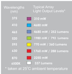
Note: Luminous output power specifications are determined by the integrated electronics, power and thermal management systems.
