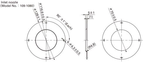
Inlet nozzle: Nozzle mounted in fan inlet side to adjust the flow of introduced air
