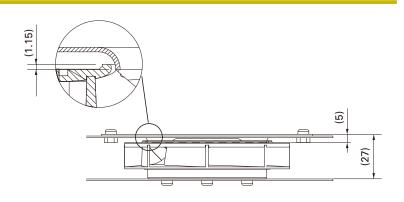
The screw length is 5mm less or equal from fan edge side.
