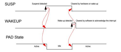
The Suspend interrupt flag (SUSP) is set and the Wake-Up interrupt flag (WAKEUP) is cleared when a USB "Suspend" state has been detected on the USB bus. This event automatically puts the USB pad in the Idle state. The detection of a non-idle event sets WAKEUP, clears SUSP and wakes up the USB pad.
