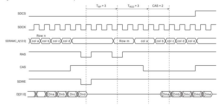
Figure 28-7. Read Burst with Boundary Row Access
