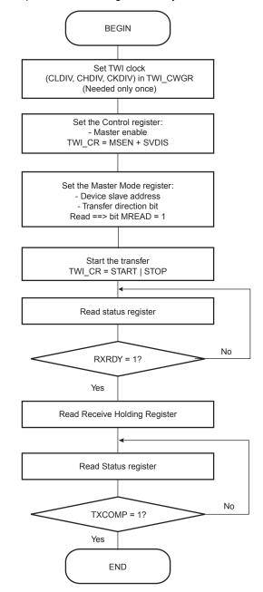
Figure 24-16. TWI Read Operation with Single Data Byte without Internal Address
