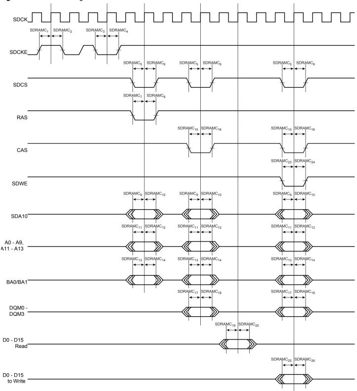
Figure 38-4. SDRAMC Signals relative to SDCK.
