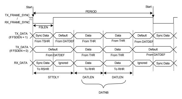
Note: 1. Example of input on falling edge of TX\_FRAME\_SYNC/RX\_FRAME\_SYNC.
