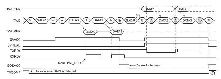
Notes: 1. In this case, if THR has not been written at the end of the read command, the clock is automatically stretched before the ACK.
