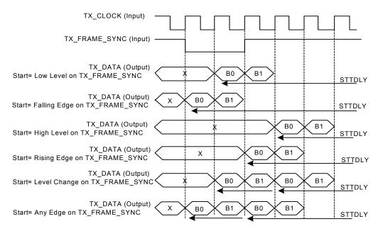
Figure 25-11. Receive Pulse/Edge Start Modes
