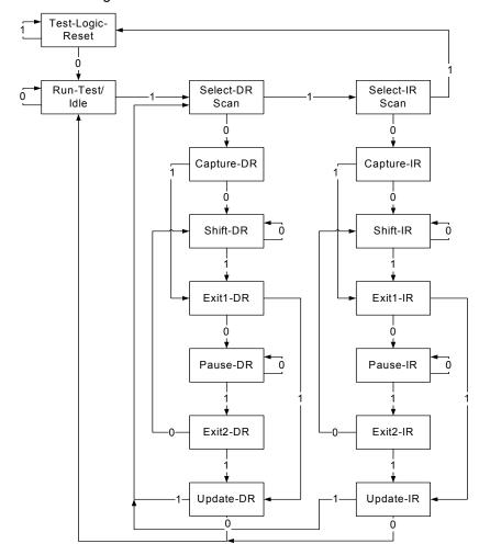
Figure 36-2. TAP Controller State Diagram
