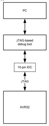
Figure 35-2. JTAG-based debugger
