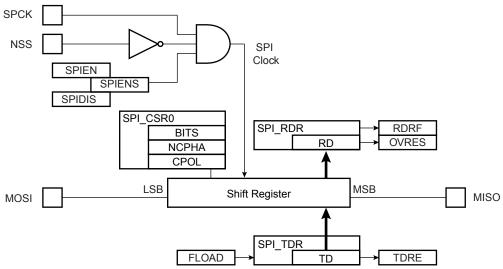
Figure 23-9. Slave Mode Functional Block Diagram
