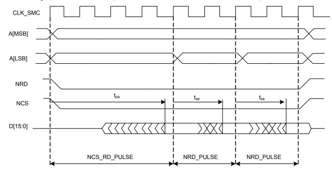
Figure 27-35. Page Mode Read Protocol (Address MSB and LSB are defined in Table 27-5)
