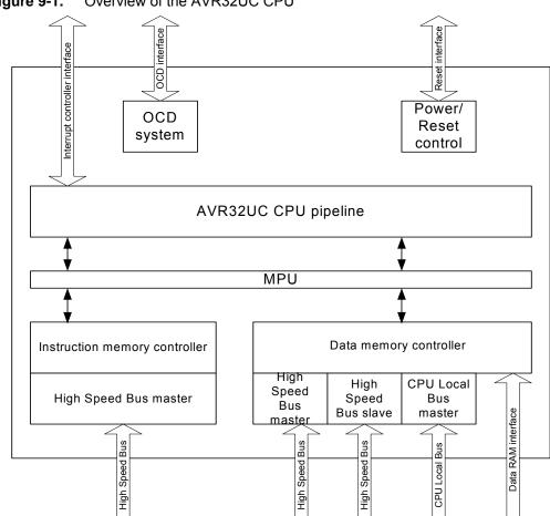
Figure 9-1. Overview of the AVR32UC CPU
