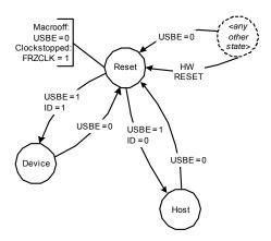
After a hardware reset, the USB controller is in the Reset state. In this state:
