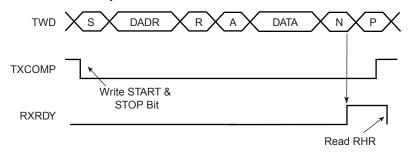
Figure 24-10. Master Read with Multiple Data Bytes
