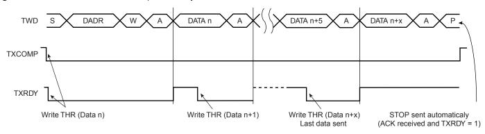
Figure 24-8. Master Write with One Byte Internal Address and Multiple Data Bytes
