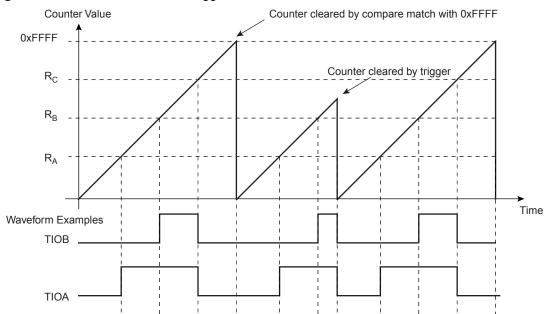
Figure 31-7. WAVSEL= 00 with trigger
