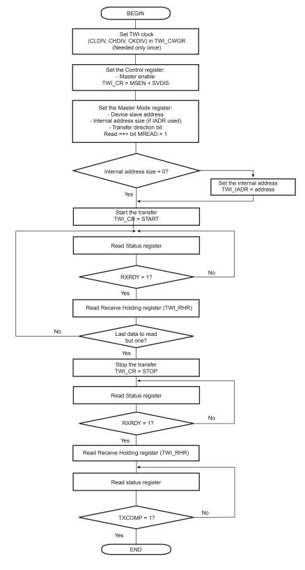
Figure 24-18. TWI Read Operation with Multiple Data Bytes with or without Internal Address
