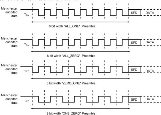
Figure 26-9. Preamble Patterns, Default Polarity Assumed
