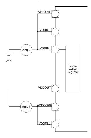
These figures represent the power consumption measured on the power supplies.
