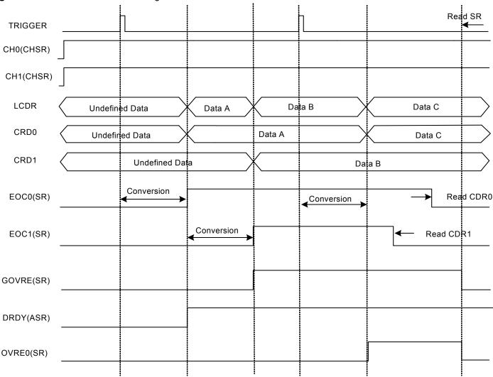
**Warning:** If the corresponding channel is disabled during a conversion or if it is disabled and then reenabled during a conversion, its associated data and its corresponding EOC and OVRE flags in SR are unpredictable.
