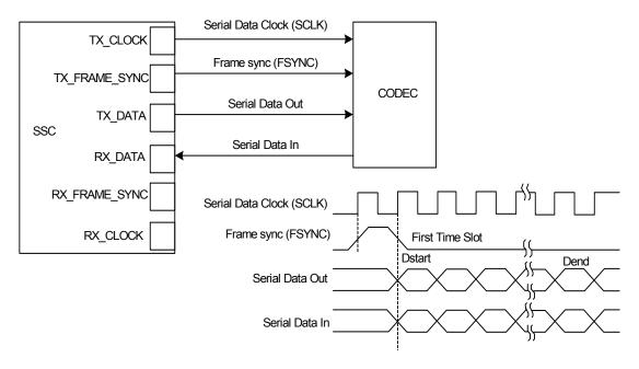
Figure 25-19. Time Slot Application Block Diagram
