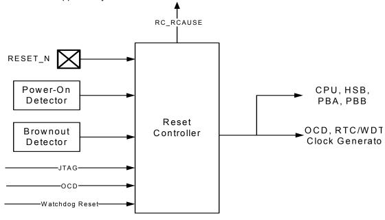
Figure 13-6. Reset Controller block diagram
