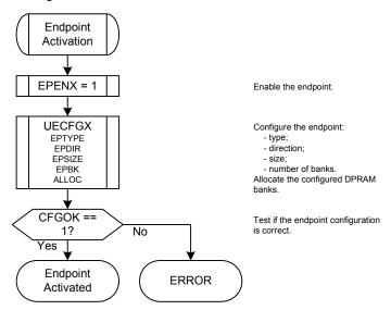
As long as the endpoint is not correctly configured (CFGOK = 0), the controller does not acknowledge the packets sent by the host to this endpoint.
