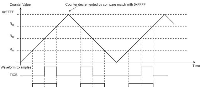
Figure 31-10. WAVSEL = 01 Without Trigger
