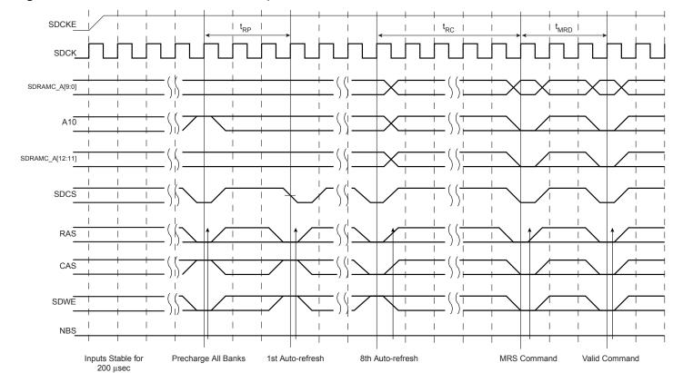
Figure 28-4. SDRAM Device Initialization Sequence
