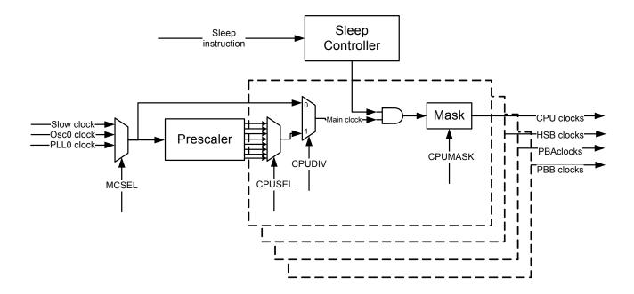
Figure 13-4. Synchronous clock generation
