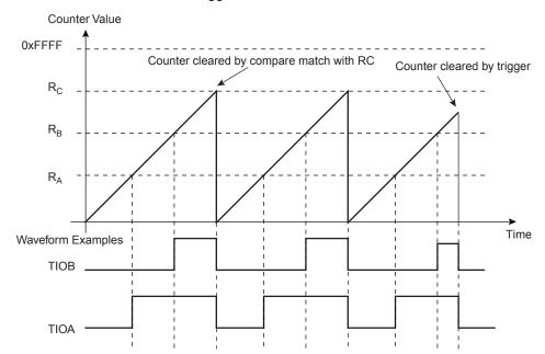
Figure 31-9. WAVSEL = 10 With Trigger
