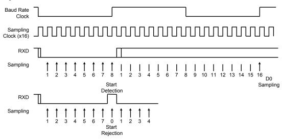
Figure 26-13. Asynchronous Character Reception
