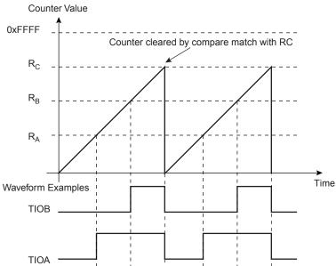
**Figure 31-8.** WAVSEL = 10 Without Trigger
