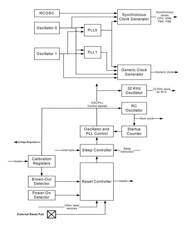
Figure 13-1. Power Manager block diagram
