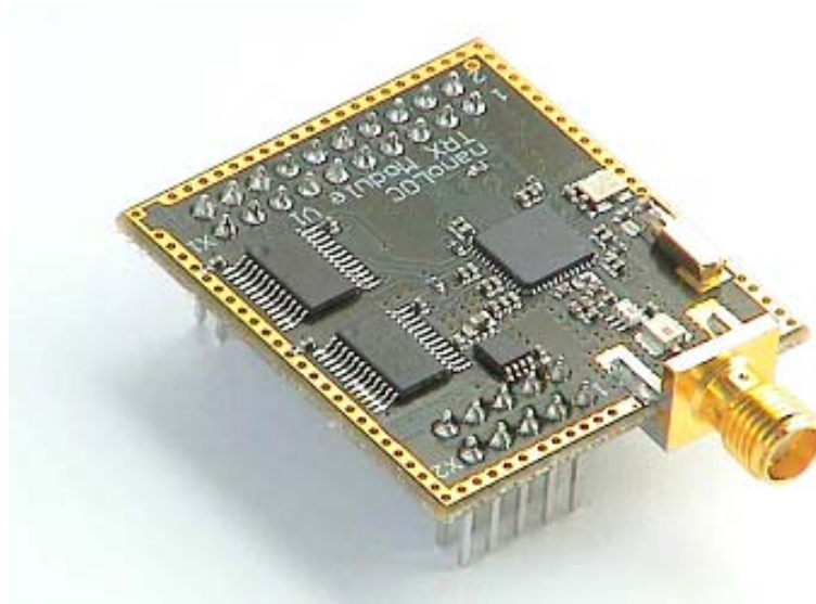
Figure 16: RF Test Module for nanoLOC chip: top view
