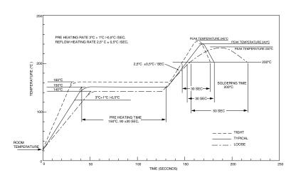
Recommended profile shown. Maximum temperature allowed on any profile is  $260^{\circ}$  C.
