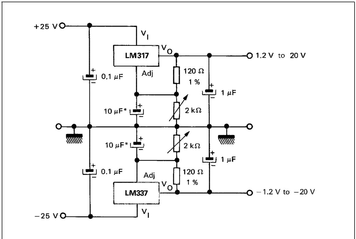
\* The 10 μF capacitors are optimal to improve ripple rejection.
