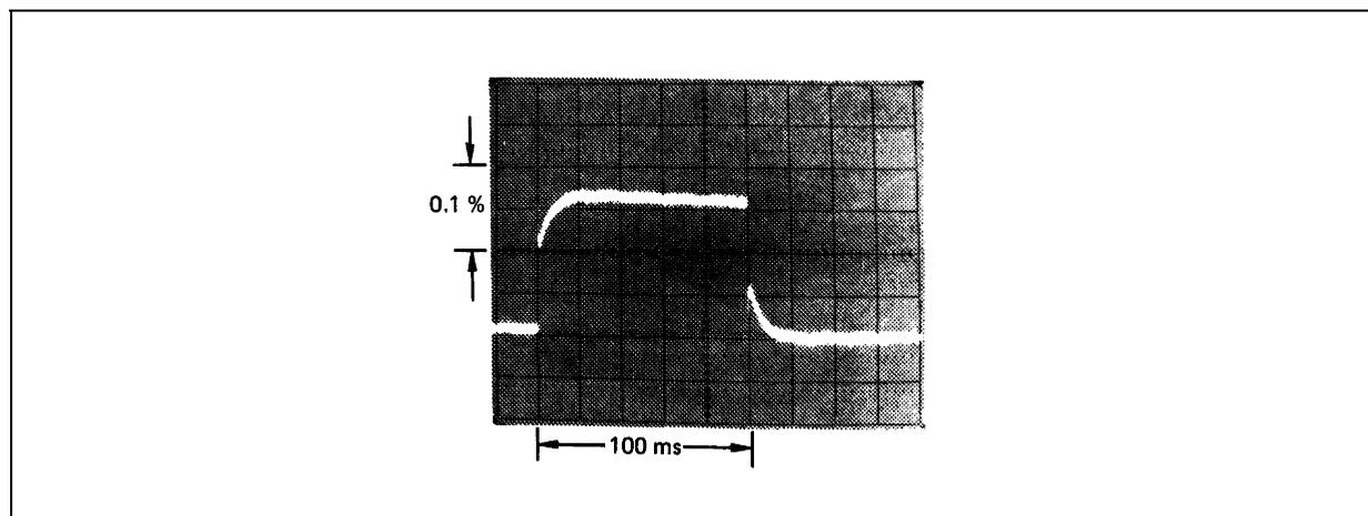
LM337,  $V_O = -10V$ ,  $V_I - V_O = -40V$ ,  $I_L = 0A \rightarrow 0.25A \rightarrow 0A$ . Horizontal sensitivity 5msN/div.
