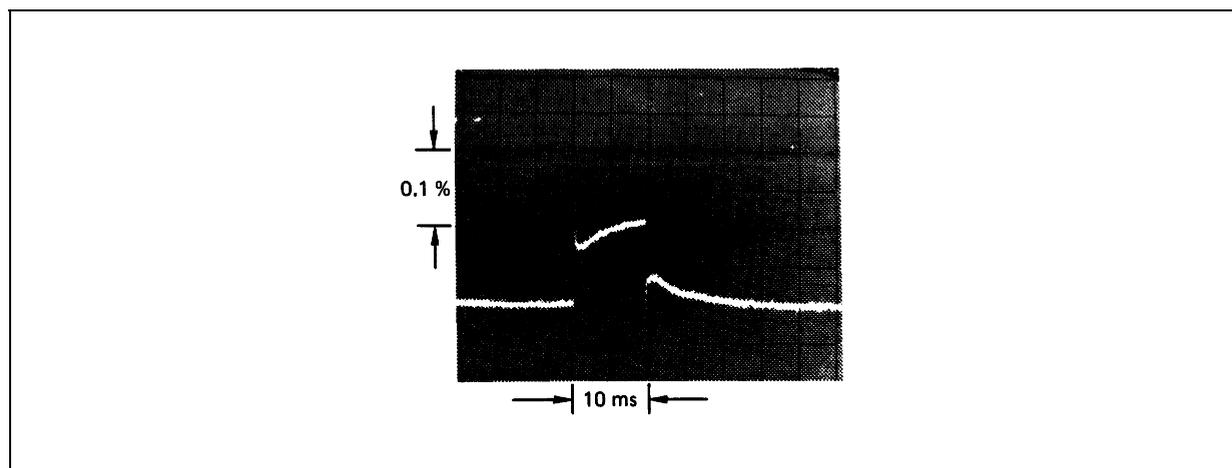
LM337,  $V_O = -10V$ ,  $V_I - V_O = -40V$ ,  $I_L = 0A \rightarrow 0.25A \rightarrow 0A$ . Vertical sensitivity 5mV/div.
