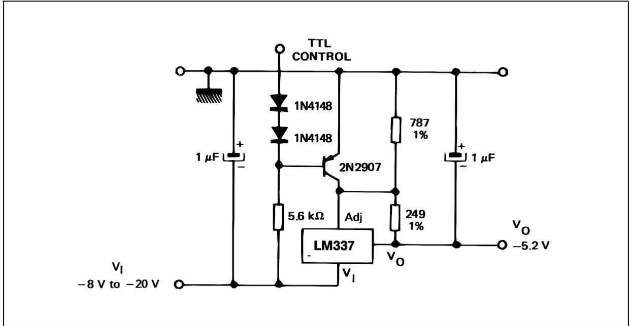
\* Minimum output = - 1.3V when control input is low.
