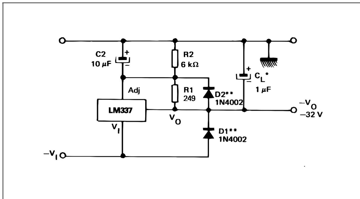
\* When  $C_L$  is larger than  $20 \mu\text{F}$ ,  $D_1$  protects the LM137 in case the input supply is shorted.
