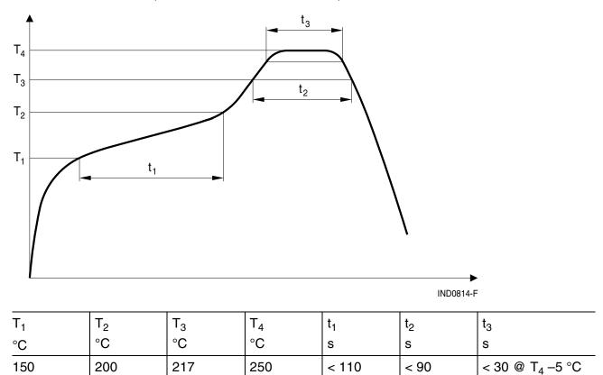
Time from 25 °C to  $T_4$ : max 300 s Maximal numbers of reflow cycles: 3 B82792C0
