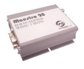
A Miniature "Plug And Play" dual band GSM modem. It can be directly connected to the serial port of a desktop or notebook computer through the RS232 interface. A standard SIM card can be inserted in the integral card holder within the metal enclosure.
