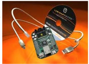
This evaluation kit enables quick evaluation, prototype development, and creation of application-specific designs for Ethernet networks. The kit also includes extensive source-code examples, allowing you to start building C-code applications quickly.
