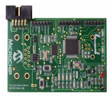
the monitor and the other one will become the Traffic Generator. The boards are reversible (i.e., they can take either role, depending on the connection scheme). Additionally, the board(s) can be connected to an existing CAN bus where the software can monitor the traffic and the user can interact with the bus as needed. The software allows some of the MCP2515 registers to be modified, as well as allows messages to be received and transmitted.
