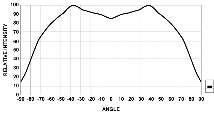
Figure 9. Relative intensity vs. angle for HSMW-C120.
