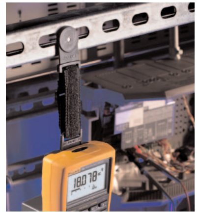
With the magnetic hangar (TPAK), you can find a convenient place to hang the compact 189 and leave it in place to log.
