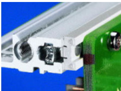
Rear horizontal rail for backplane assembly
