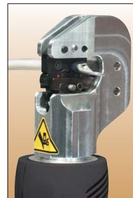
Uses the exact dies of the Comfort Crimp line of ergonomic tools for Sta-Kon, Spec-Kon, and Dragon Tooth.
