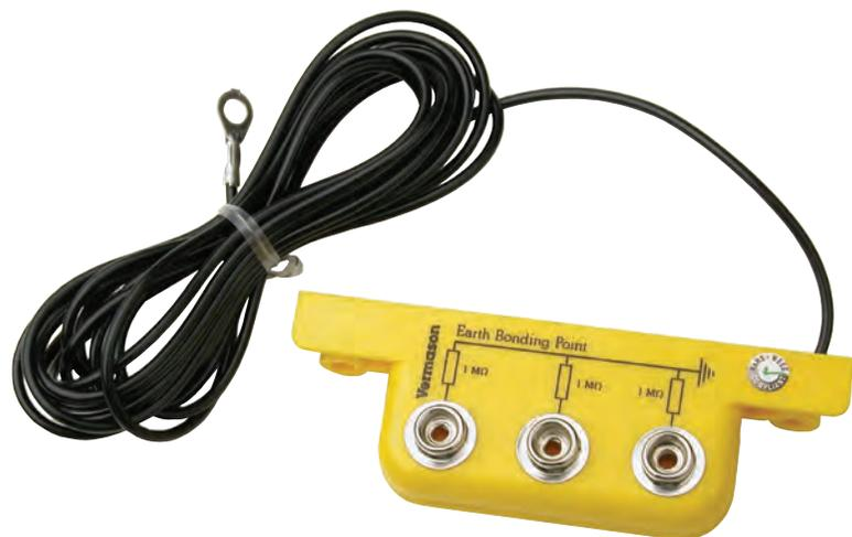
"The protection of ESDS [ESD sensitive item] is accomplished by providing a ground path to bring ESD protective materials and personnel to the same electrical potential. All conductor and dissipative items in the environment, including personnel, shall be bonded or electrically connected to a known ground or common connection point [Earth Bonding Point]." [CLC/TR 61340-5-2 User guide clause 4.4.1 Grounding/bonding systems Introduction]
