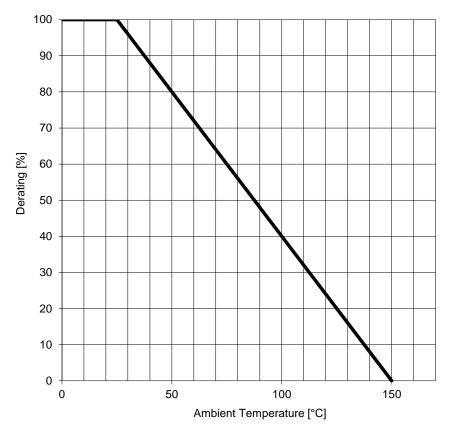
**Steady State Power Dissipation Derating:**
