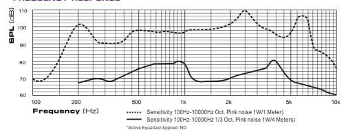
GB20T/EN & GB20T/ENC has been tested in 100 hours max power (10W). The model does not deviate by more than ± 3dB from the original test value. The frequency response curve and impedance complies with the original one. All SPL tests are performed in an anechoic chamber (<70m³)
