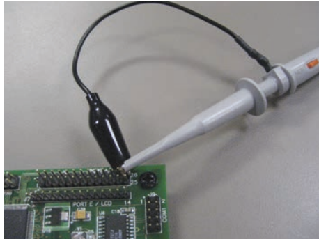
Figure 6-1. Connect both probe tips to the ground and see if any signals appear on the screen.
