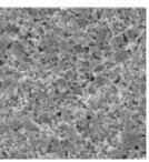
• **Silver** offers the best shielding and corrosion resistance. It is also the best choice for board level shielding and mission critical applications. It can be applied very thinly.
