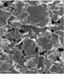
• **Silver-coated copper** provides superior shielding at higher frequencies.
