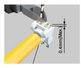
Step 3: Trim excess wires. The tips of the wires should protrude no more than 0.4mm.
