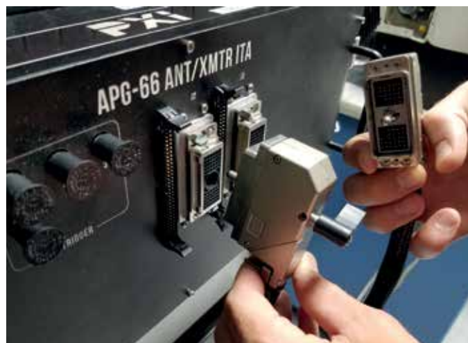
Figure 1: The cam in this test rack is easy to engage with the lever. For tight spaces, the lever can be replaced to move the cam. Another option is a self-actuated cam that, for example can mate and unmate when a drawer is closed or opened. (Learn more at Duotechservices.com )
