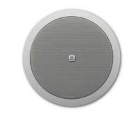
The CM20T two-way built-in loudspeaker can be used as a 16 ohms or 100 volt loudspeaker. In 16 ohms use, you can connect up to 4 loudspeakers in parallel on each channel of a standard 4 ohms amplifier. For 100 volt use, the CM20T is equipped with a high-quality 20 watts 100 volt transformer with several power tappings (20 - 10 - 5 - 2.5 watts). Therefore it can be used in projects with high ceilings or places with background noise where a little more power is needed.
