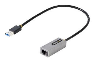
Easily add a Gigabit network port to your computer through a USB 3.0/3.2 Gen 1 Type-A port. The RJ45 port supports multiple speeds (10/100/1000 Mbps) and is fully compatible with Cat5, Cat5e, Cat6, and Cat6a cabling. This is an ideal peripheral for newer laptops that don't have an Ethernet port anymore. With backward compatibility, add network capabilities to older computers or replace a non-working Ethernet port.
