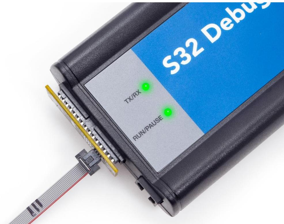
Figure 10. S32 Debug Probe - LED indicators
