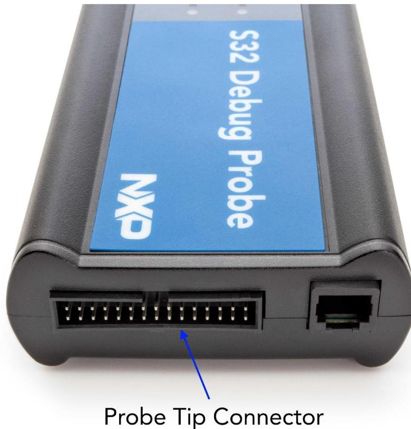
Figure 13. S32 Debug Probe - target side view
