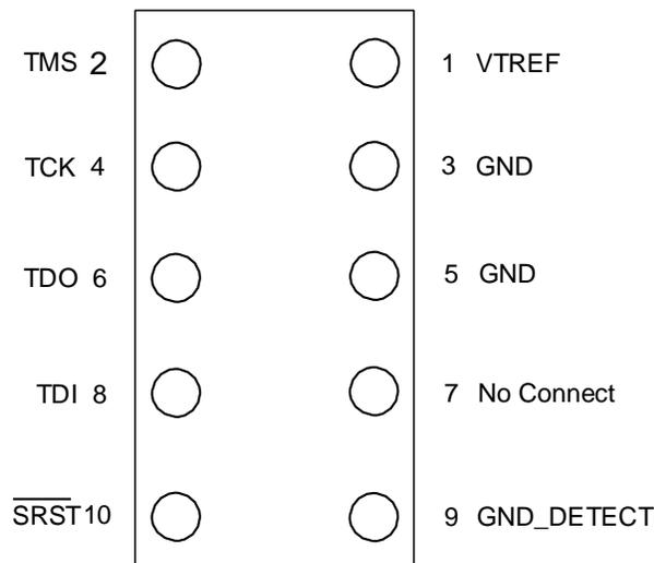
Figure 20. S32 Debug Probe for Arm connector pin assignments Table
