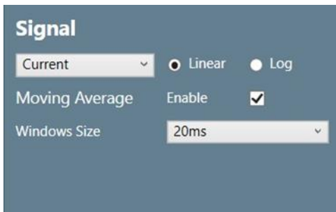
Figure 3-7 Controls to select signal to show, switch between linear and logarithmic display as well as optional moving filter enabled for 20 ms averaging time to suppress remaining 50 Hz noise
