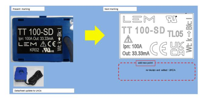
The new marking will still be on black background sheet with text in white color as the current one. Here above illustrations show the new marking information layout on the label. But the color of label and text with new marking will be the same as with the current label.
