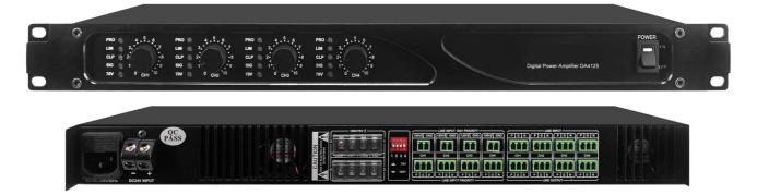
ADS DA4125 4 x 125watts and ADS DA4250 4 x 250watt, rack mount 1U Class D 100V digital amplifiers are for commercial and industrial public address applications. Balanced & unbalanced line inputs for each channel. Balanced line output for connection to additional power amplifier
