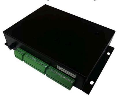
The DMP20 is a rugged industrial WAV player designed for the most demanding jobs. Much like a CD player playing sound tracks from a CD, DMP20 plays sound files from an SD/SDHC memory card but without the moving parts to wear and tear. The file format support is 8-bit uncompressed WAV files with sampling rate up to 22.05KHz.
