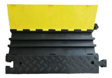
A heavy duty, 3 channel cable protector which interlinks to form a continuous ramped cable protector. The highly visible yellow hinged lid allows cables to be inserted after the ramps are in position and each section has fixing holes provided for optional permanent fixing.
