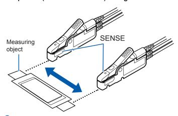
3 Adjust the position of the probes such that the return cable between the probes does not sag, and fix by pushing the return cable into the grooves of the probes.
