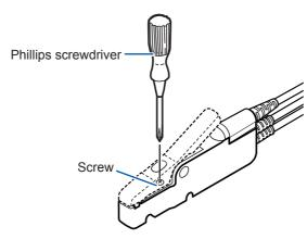
Adjust the stopper position by moving the stopper back and forth and tighten the screw.
