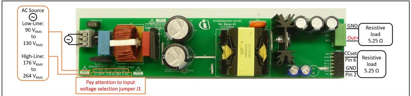
**Figure 3** EMI test setup with full output power
