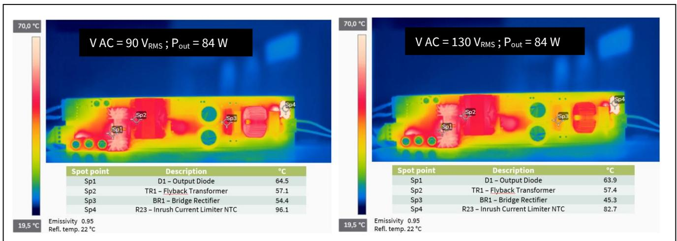
Figure 15 IR thermal image of PCB top components at low-line input
