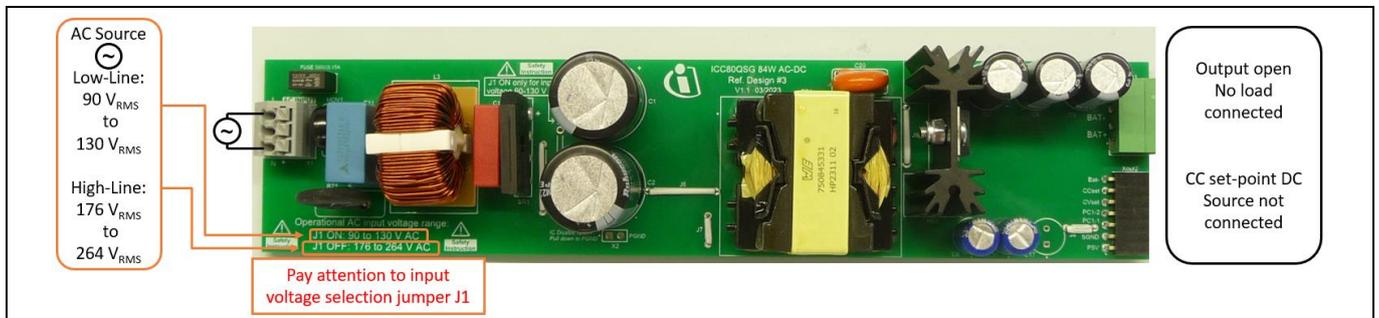
**Figure 4** No-load system standby power test setup
