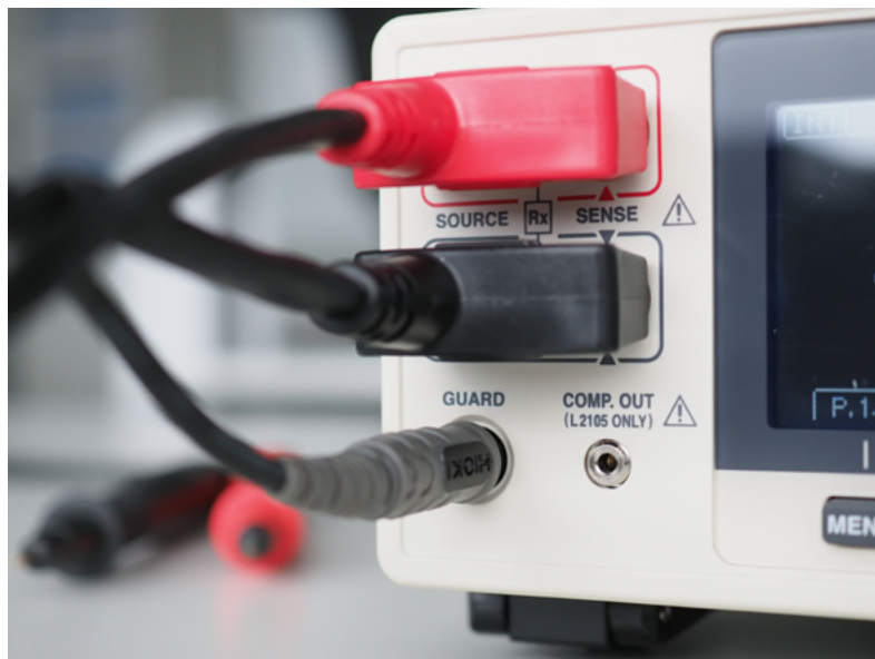
Figure 4: Guard terminal: More stable measurements in high resistance ranges
