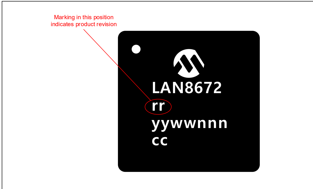
FIGURE 3: TOP MARKING FOR LAN8672 DEVICE
